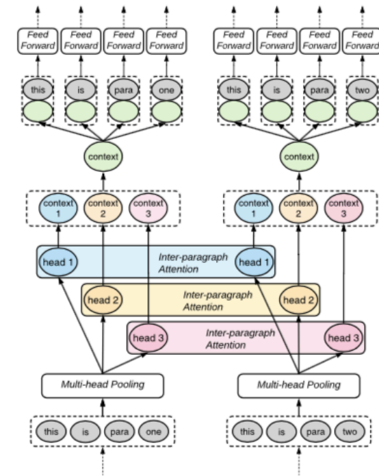
Figure 2: A global transformer layer. Different colors indicate different heads in multi-head pooling and inter-paragraph attention.
